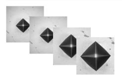
Calibrated stepless zoom of the indent image provided by the objective, while maintaining the same high standard of image quality. This unique zoom system is a standard feature on the entire FALCON series.
