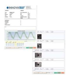
The IMPRESSIONS<sup>TM</sup> system incorporates a very advanced report generator. The report generator allows you to publish all testing results and graphics, including pictures of the indentations in an easy to edit and easy to customize file size. You can add your company details and change the reporting lay-out to your requirements.
