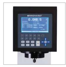
NEXUS 3001XLM-IMP can also be operated as a Brinell indentation press only. Without the use of the IMPRESSIONS<sup>™</sup> interface.
